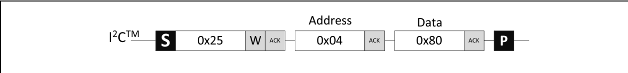
FIGURE 5-3: EXAMPLE I 2 C™ READ TRANSACTION
