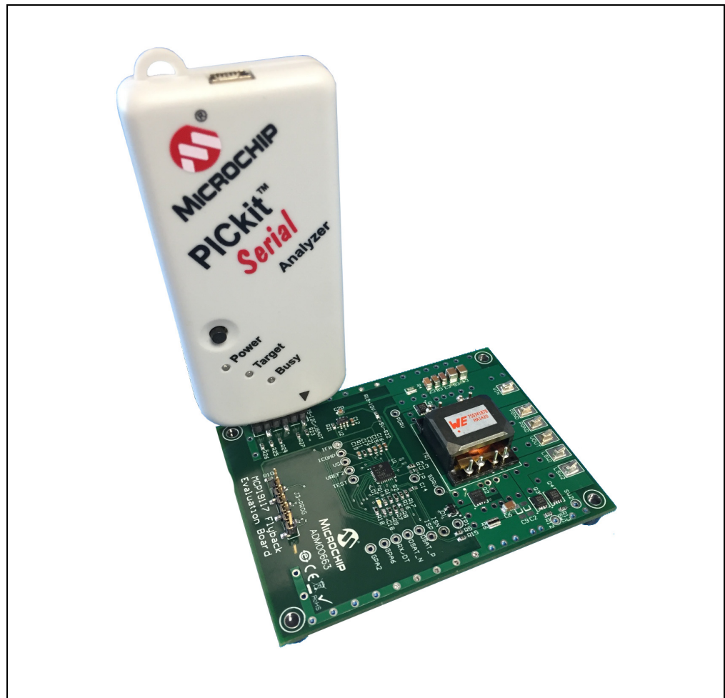
FIGURE 3-1: PICkit Serial Analyzer Connection to the Board.
