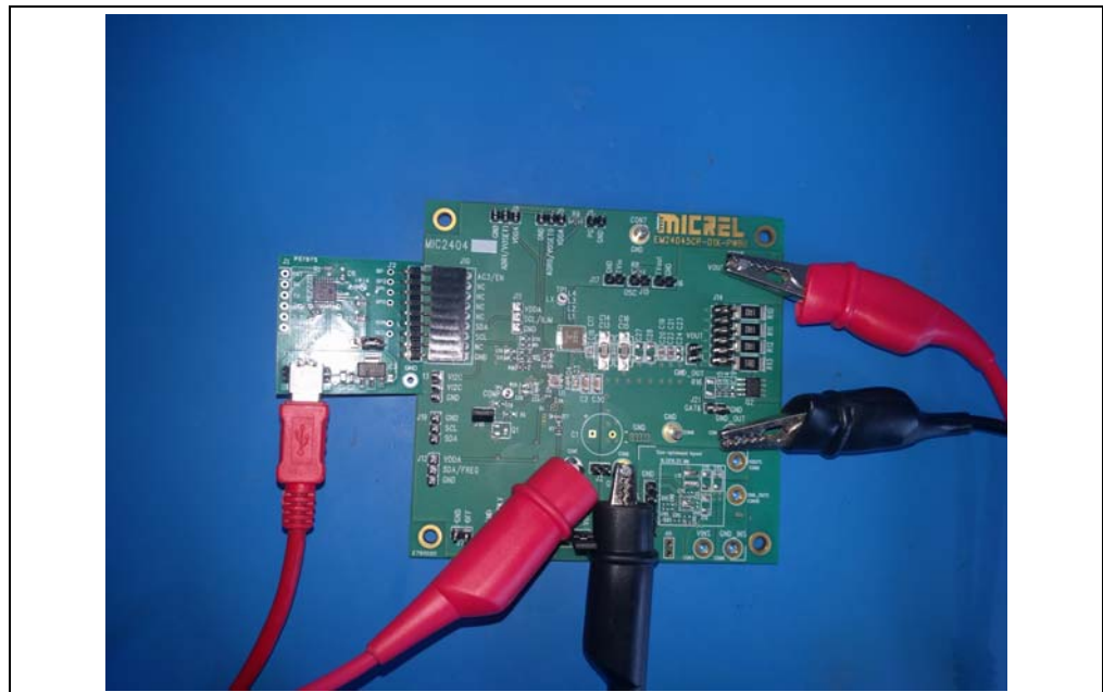
FIGURE 2-1: MIC24045 with MCP2221 Board Connection.
