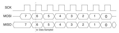
Figure 24-10. Serial Programming Interface Timing
