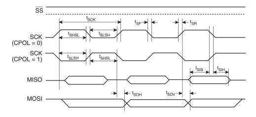
Figure 25-16. SPI Slave Timing (CPHA = 1)
