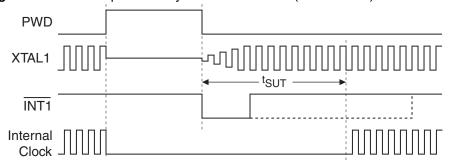
When PWDEX = "1", the wake-up period is controlled externally by the interrupt. Again, at the falling edge on the interrupt pin, power-down is exited and the oscillator is restarted. However, the internal clock will not propagate until the rising edge of the interrupt pin as shown in Figure 11-2. The interrupt pin should be held low long enough for the selected clock source to stabilize. After the rising edge on the pin the interrupt service routine will be executed.
