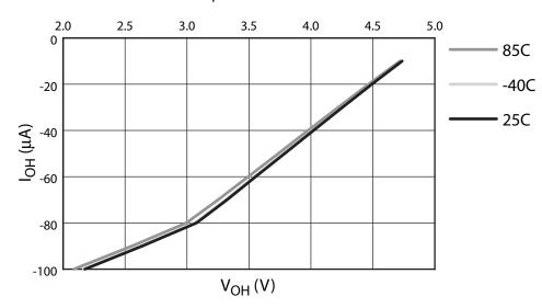
Figure 25-7. Quasi-Bidirectional Output I-V Characteristic at 3V
