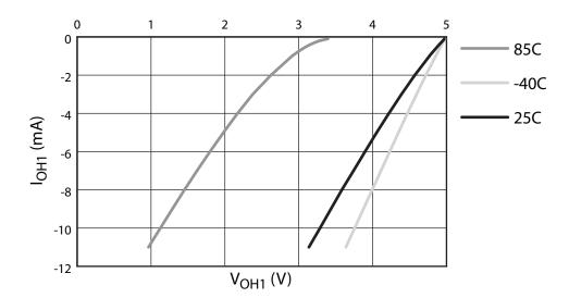
Figure 25-9. Push-Pull Output I-V Characteristic at 3V
