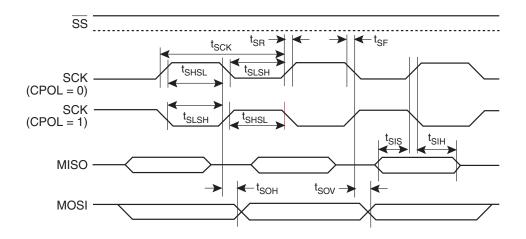
Figure 25-14. SPI Slave Timing (CPHA = 0)
