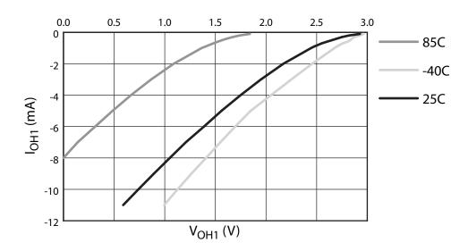
Note: Under DC operating conditions the Push-Pull Outputs exhibit reduced V<sub>OH</sub> levels at higher temperatures due to the 5V tolerant port structure. Under AC conditions a boost circuit provides additional source current. If additional DC source current is required, or if V<sub>OH</sub> is too low, external pull-ups may be needed. DC conditions are most likely to exist when the device enters Powerdown mode.
