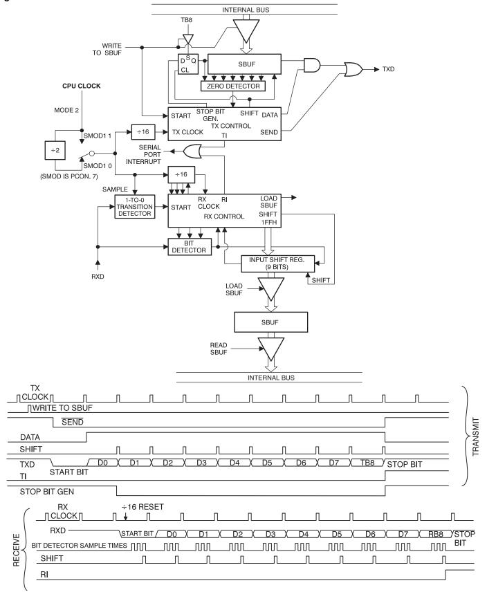
Figure 18-4. Serial Port Mode 3
