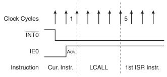
Figure 12-2. Maximum Interrupt Response Time
