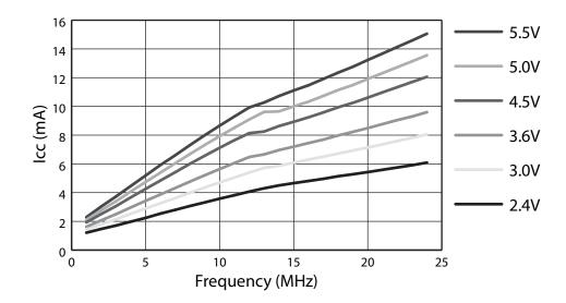
Figure 25-4. Idle Supply Current vs. Frequency
