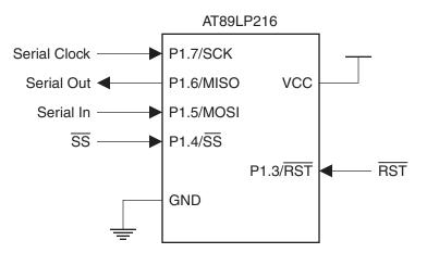
The In-System Programming Interface is the only means of externally programming the AT89LP216 microcontroller. The ISP Interface can be used to program the device both in-system and in a stand-alone serial programmer. The ISP Interface does not require any clock other than SCK and is not limited by the system clock frequency. During In-System programming the system clock source of the target device can operate normally.
