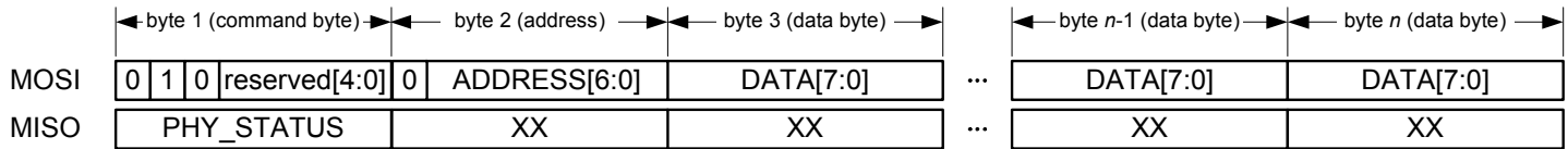
Figure 6-12. Packet Structure - SRAM Write Access
