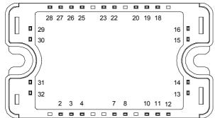
All multiple inputs and outputs must be shorted together Example: 10/11/12; 7/8 ...
