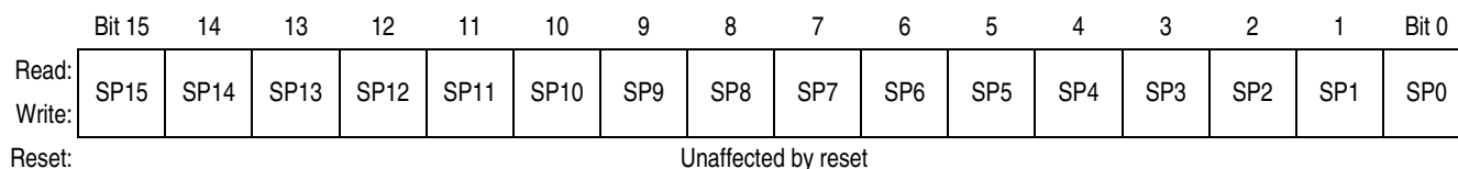
Figure 3-7. Stack Pointer (SP)
