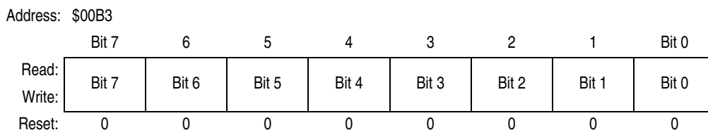
Figure 13-47. 8-Bit Pulse Accumulator Holding Register 2 (PA2H)
