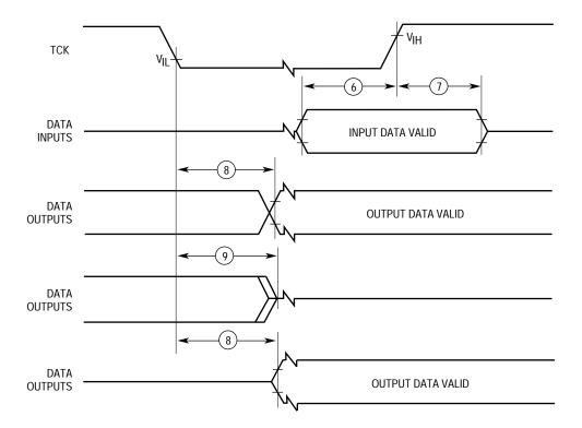
Figure 11-20. Boundary Scan Timing Diagram
