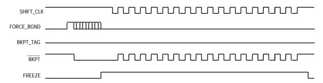
Figure 5-25. BKPT Timing for Forcing BDM
