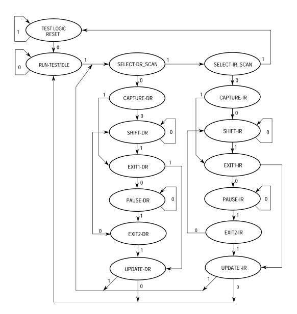
Figure 9-2. TAP Controller State Machine
