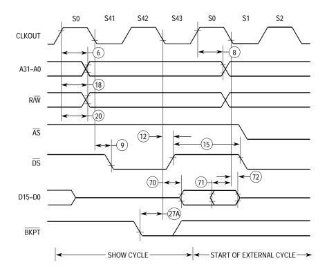
Figure 11-8. Show Cycle Timing Diagram
