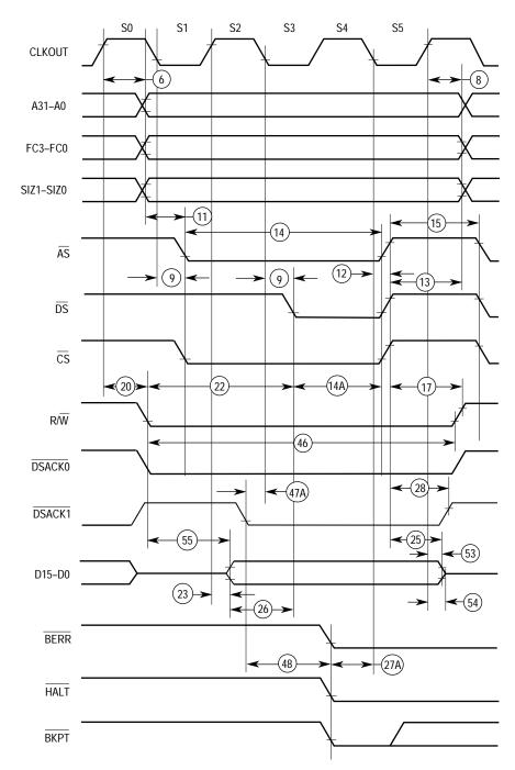
NOTE: All timing is shown with respect to 0.8-V and 2.0-V levels.
