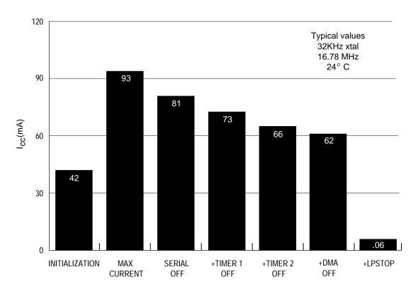
Figure 10-15. MC68340 Current vs. Activity at 5 V
