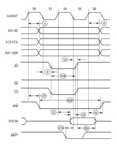
Figure 11-5. Fast Termination Write Cycle Timing Diagram
