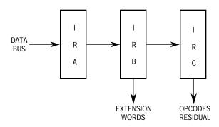
Figure 5-28. Functional Model of Instruction Pipeline
