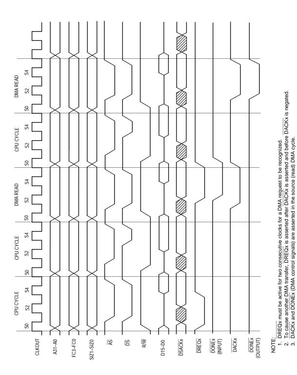
Figure 6-6. Single-Address Read Timing (Cycle Steal)
