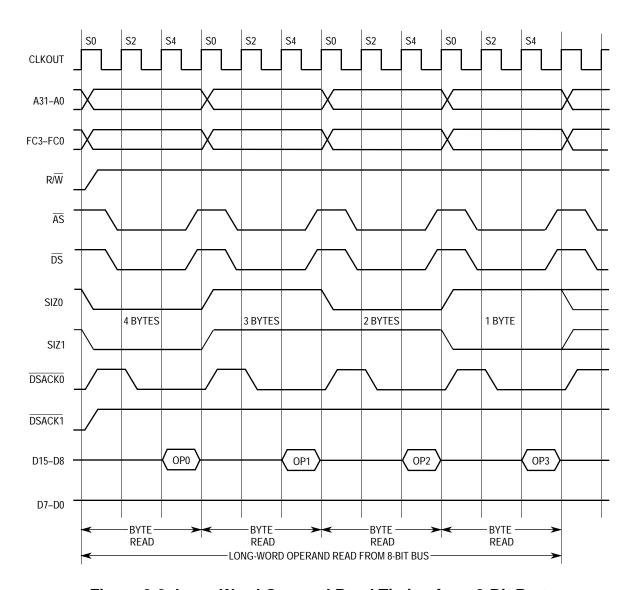
Figure 3-3. Long-Word Operand Read Timing from 8-Bit Port
