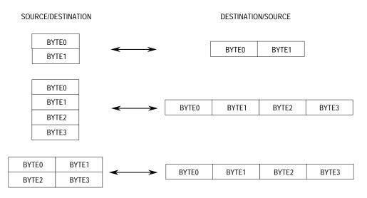
Figure 6-16. Packing and Unpacking of Operands
