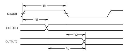
Figure 10-13. Skew between Two Outputs
