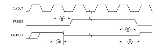
Figure 11-11. Background Debug Mode FREEZE Timing
