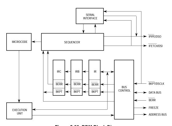
Figure 5-20. BDM Block Diagram
