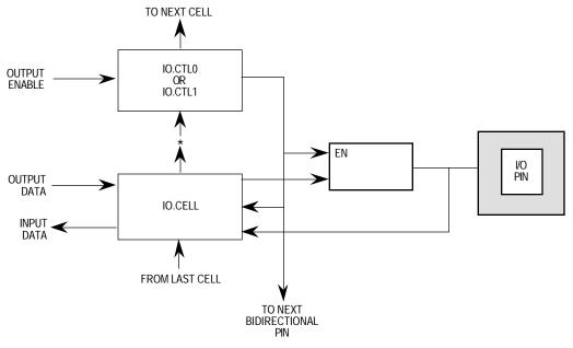
NOTE: More than one IO.Cell could be serially connected and controlled by a single IO.Ctlx cell.
