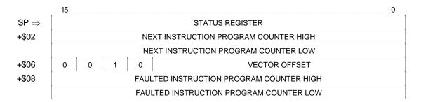
Figure 5-13. Format \$2—Six-Word Stack Frame
