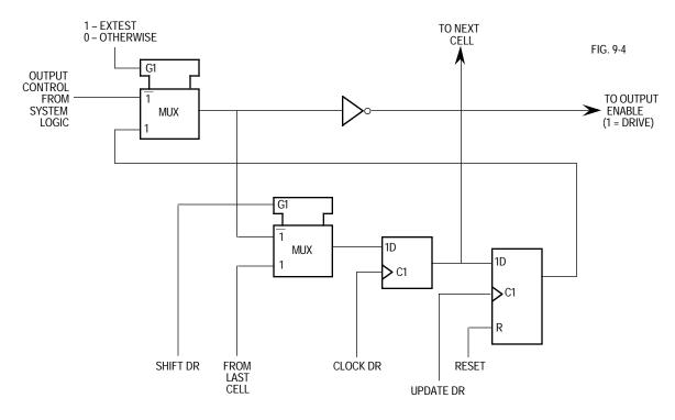
Figure 9-6. Active-Low Output Control Cell (IO.Ctl0)
