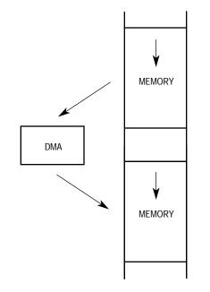
Figure 6-3. Dual-Address Transfer
