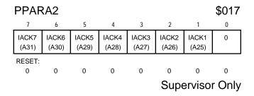
The IACK≈ signals are asserted if a bit in PPARA2 is set and the CPU32 services an external interrupt at the corresponding level. IACK≈ signals have the same timing as address strobes.
