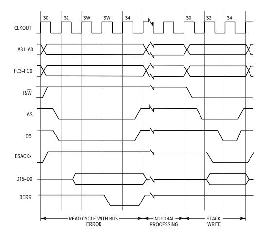
Figure 3-17. Bus Error without DSACK≈
