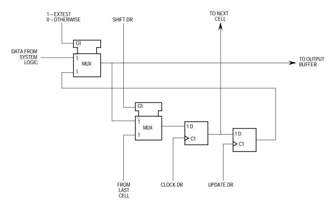
Figure 9-3. Output Latch Cell (O.Latch)
