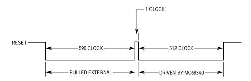
Figure 3-27. Timing for External Devices Driving RESET
