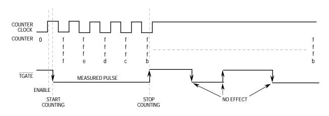
MODEx Bits in Control Register = 100 TGE Bit of Control Register = 1
