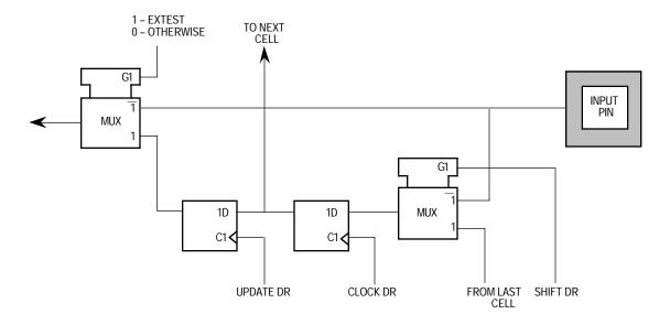
Figure 9-4. Input Pin Cell (I.Pin)
