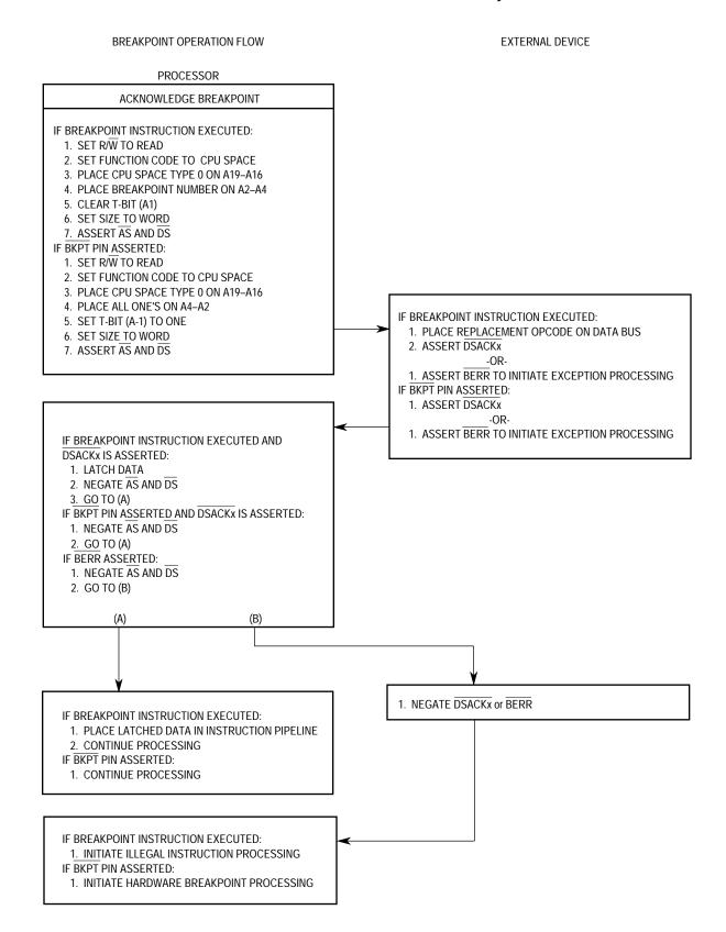
Figure 3-11. Breakpoint Operation Flowchart
