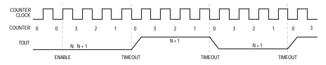
MODEx Bits in Control Register = 001 Preload 1 Register = N = 3 OCx Bits in Control Register = 01
