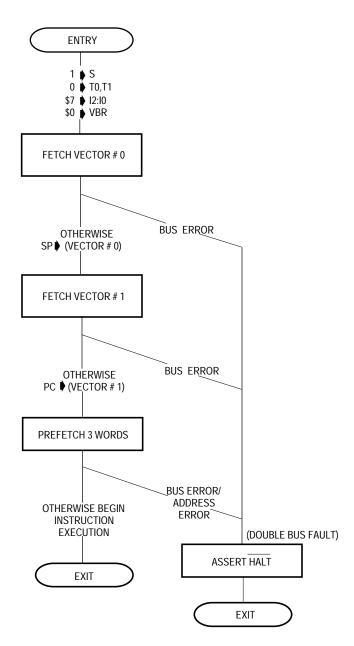
Figure 5-11. Reset Operation Flowchart
