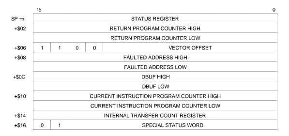
Figure 5-16. Format \$C—BERR Stack on MOVEM Operand
