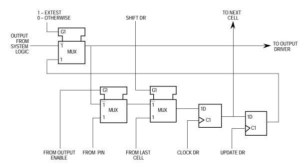
Figure 9-7. Bidirectional Data Cell (IO.Cell)
