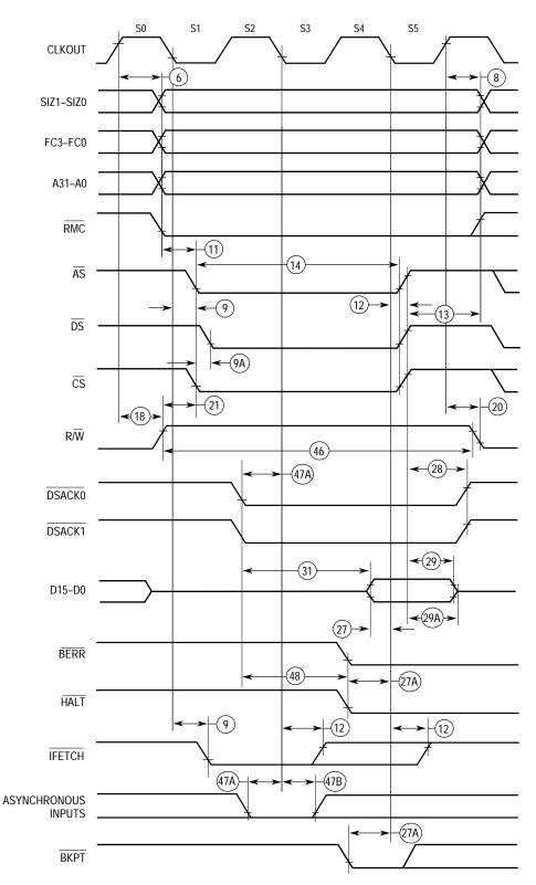
NOTE: All timing is shown with respect to 0.8V and 2.0V levels.
