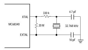
Figure 10-2. Sample Crystal Circuit
