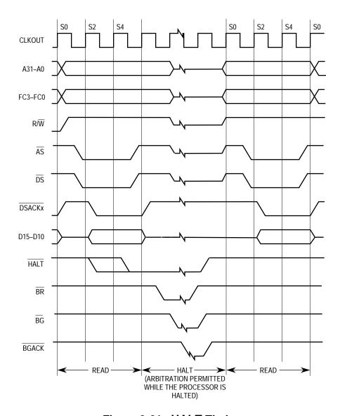
Figure 3-21. HALT Timing
