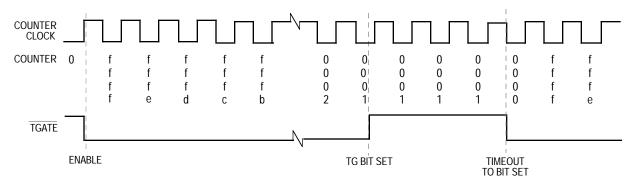
MODEx Bits in Control Register = 110 TGE Bit of the Control Register = 1
