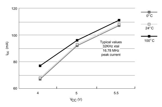
Figure 10-16. MC68340 Current vs. Voltage/Temperature
