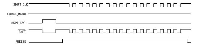
Figure 5-24. BKPT Timing for Single Bus Cycle
