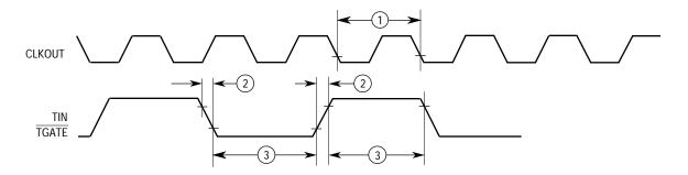
Figure 11-13. Timer Module Clock Signal Timing Diagram
