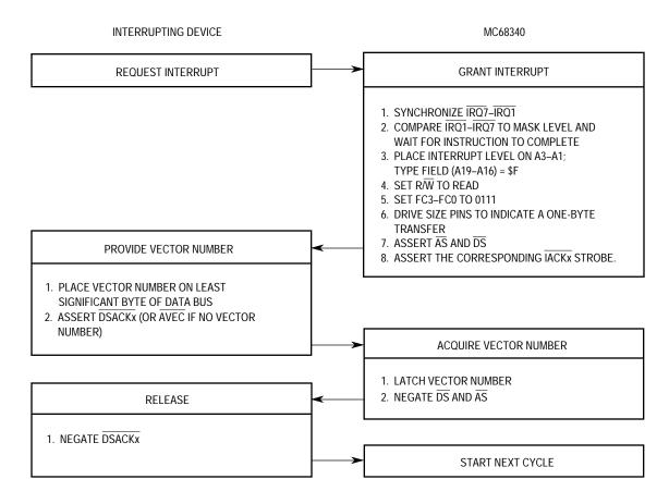
Figure 3-14. Interrupt Acknowledge Cycle Flowchart
