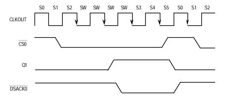
Figure 10-9. 8-bit Boot ROM Timing
