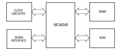
Figure 10-1. Minimum System Configuration Block Diagram
