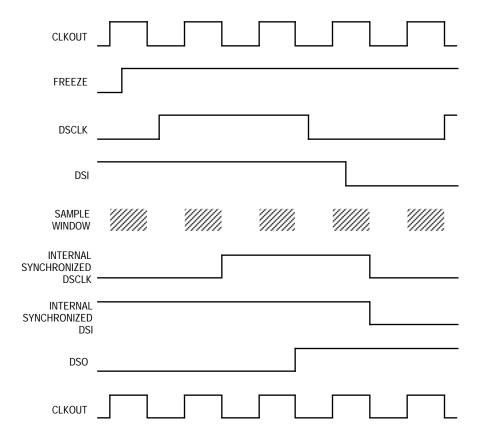
Figure 5-23. Serial Interface Timing Diagram
