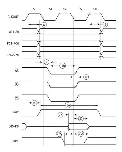
Figure 11-4. Fast Termination Read Cycle Timing Diagram
