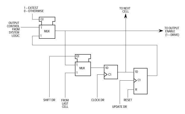
Figure 9-5. Active-High Output Control Cell (IO.Ctl1)
