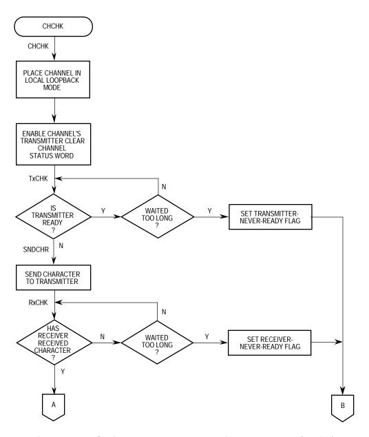
Figure 7-10. Serial Module Programming Flowchart (2 of 5)
