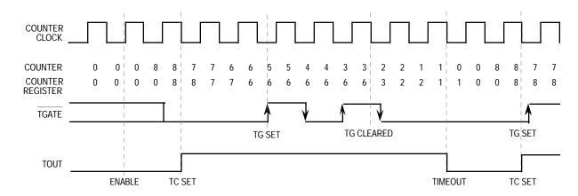
Modex Bits in Control Register = 000 Preload 1 Register = 8 Compare Register = 7 TGE Bit of Status Register = 1 TG Bit in Status Register Initially = 0 OCx Bits in Control Register = 10
