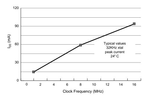
Figure 10-17. MC68340 Current vs. Clock Frequency at 5 V
