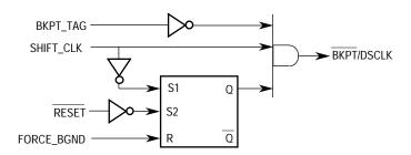
Figure 5-26. BKPT/DSCLK Logic Diagram
