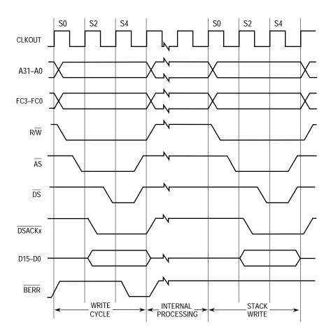
Figure 3-18. Late Bus Error with DSACK≈
