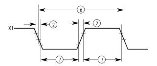
Figure 11-16. Serial Module Asynchronous Mode Timing (X1)
