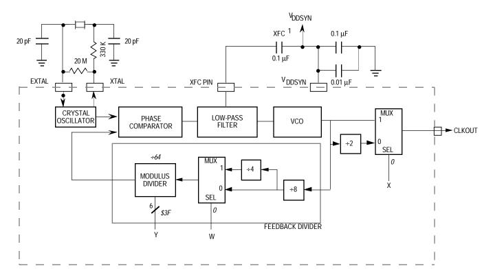
NOTE 1: Must be low-leakage capacitor.
