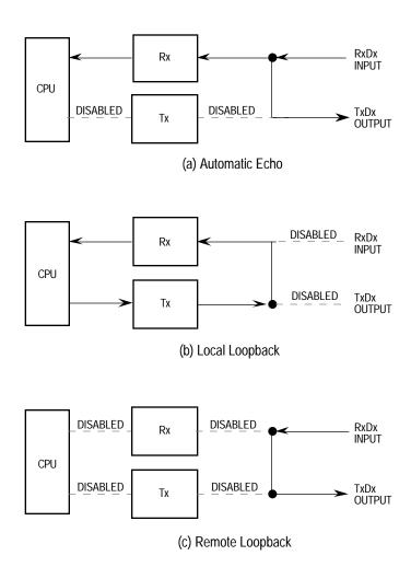
Figure 7-7. Looping Modes Functional Diagram
