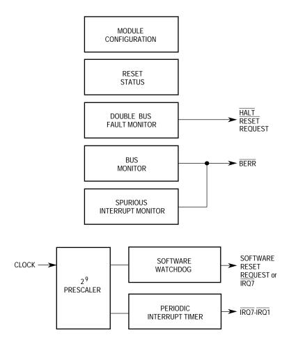
Figure 4-2. System Configuration and Protection Function
