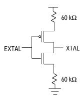
Figure 4-5. MC68340 Crystal Oscillator
