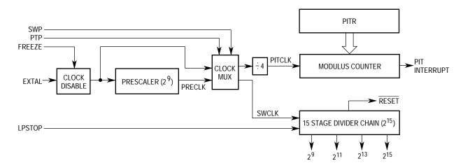
Figure 4-3. Software Watchdog Block Diagram
