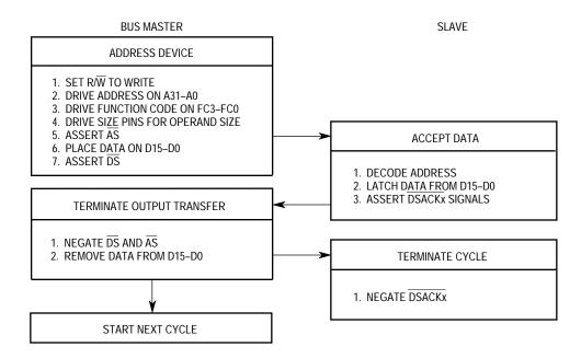
Figure 3-8. Word Write Cycle Flowchart
