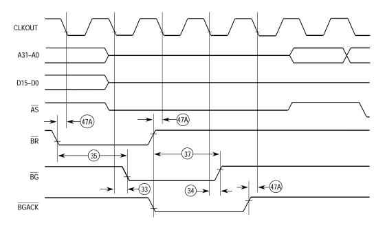
Figure 11-7. Bus Arbitration Timing—Idle Bus Case
