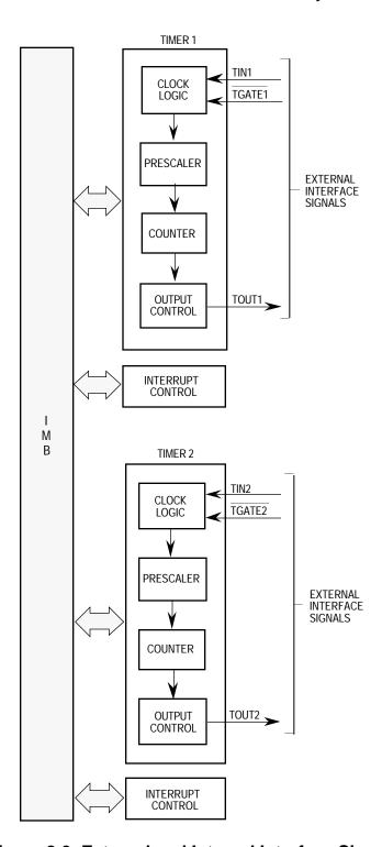
Figure 8-3. External and Internal Interface Signals
