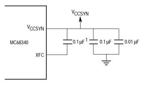
NOTE 1: Must be a low-leakage capacitor.
