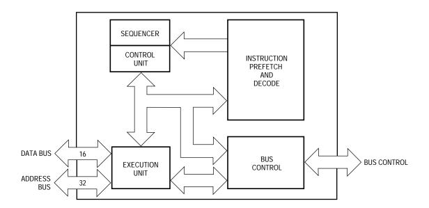
Figure 5-1. CPU32 Block Diagram
