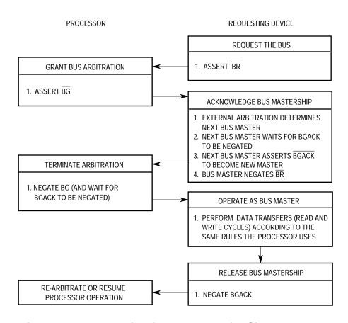
Figure 3-22. Bus Arbitration Flowchart for Single Request
