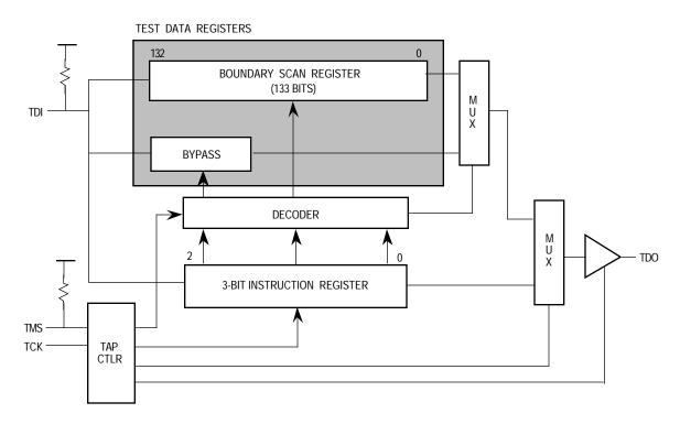
Figure 9-1. Test Access Port Block Diagram
