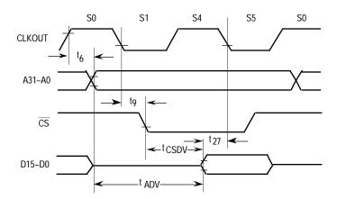
Figure 10-10. Access Time Computation Diagram
