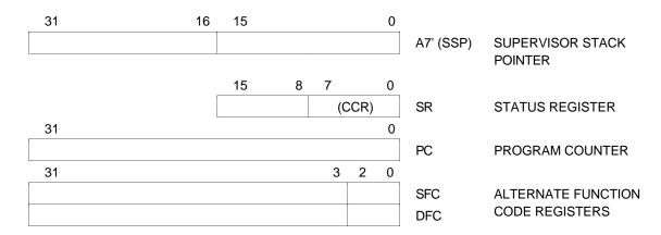
Figure 5-4. Supervisor Programming Model Supplement
