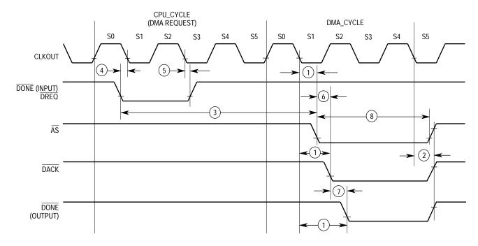
Figure 11-12. DMA Signal Timing Diagram
