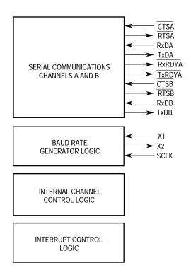
Figure 7-1. Simplified Block Diagram
