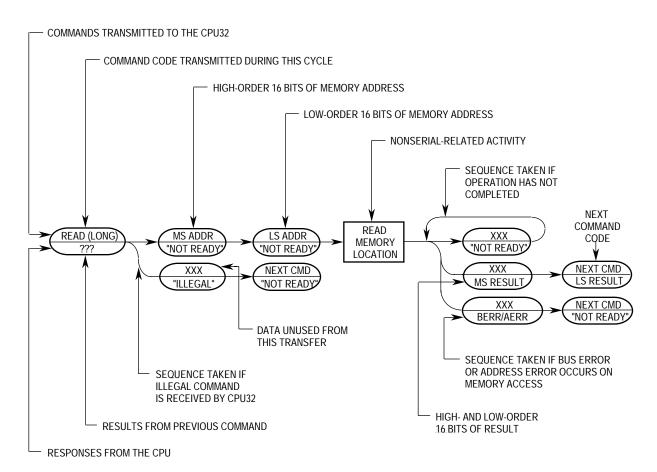
Figure 5-27. Command-Sequence Diagram
