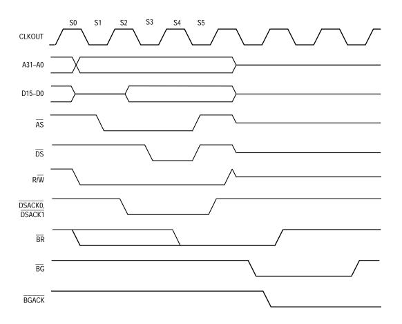
Figure 3-24. Bus Arbitration Timing Diagram—Active Bus Case
