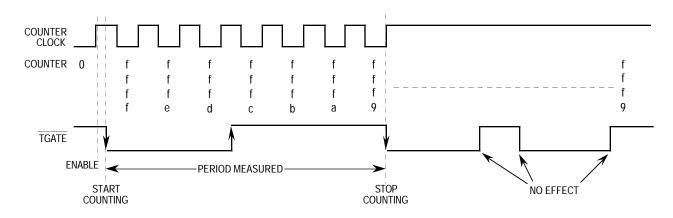
MODEx Bits in Control Register = 101 TGE Bit of Control Register = 1
