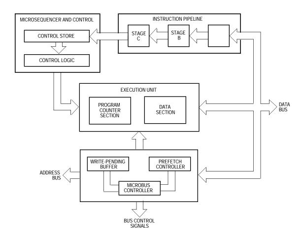
Figure 5-30. Block Diagram of Independent Resources
