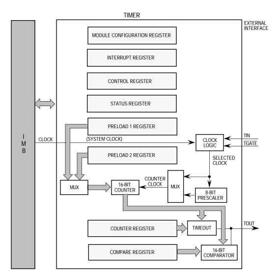
Figure 8-2. Timer Functional Diagram
