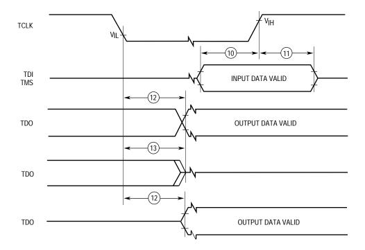
Figure 11-21. Test Access Port Timing Diagram
