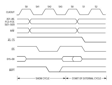
Figure 3-26. Show Cycle Timing Diagram
