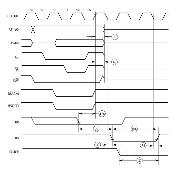
Figure 11-6. Bus Arbitation Timing—Active Bus Case
