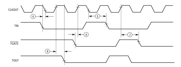
Figure 11-14. Timer Module Signal Timing Diagram
