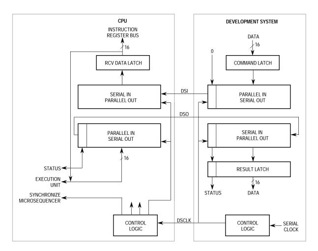
Figure 5-22. Debug Serial I/O Block Diagram
