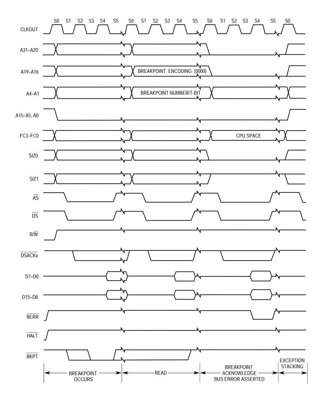
Figure 3-13. Breakpoint Acknowledge Cycle Timing (Exception Signaled)
