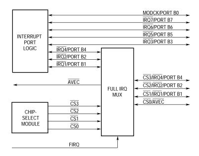
Figure 4-7. Full Interrupt Request Multiplexer
