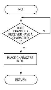
Figure 7-10. Serial Module Programming Flowchart (4 of 5)
