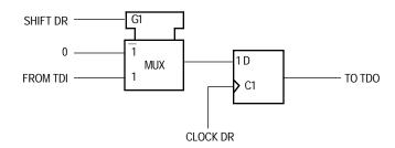
Figure 9-9. Bypass Register
