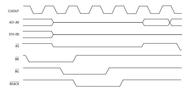
Figure 3-23. Bus Arbitration Timing Diagram—Idle Bus Case
