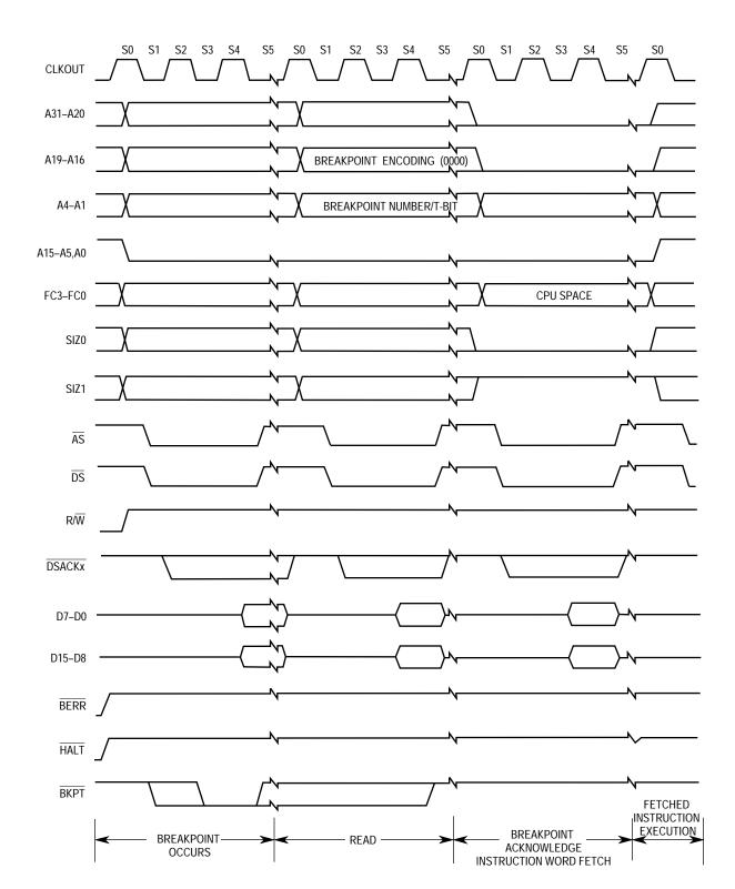
Figure 3-12. Breakpoint Acknowledge Cycle Timing (Opcode Returned)
