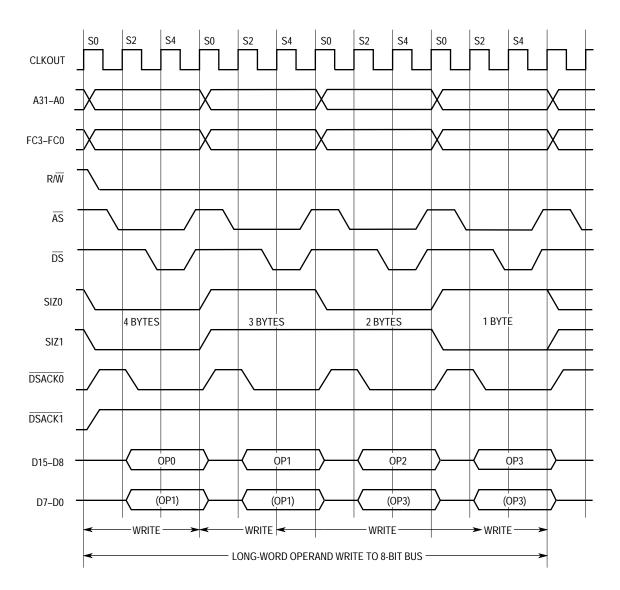
Figure 3-4. Long-Word Operand Write Timing to 8-Bit Port
