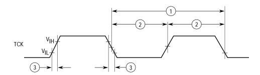
Figure 11-19. Test Clock Input Timing Diagram
