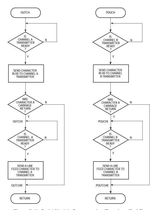
Figure 7-10. Serial Module Programming Flowchart (5 of 5)
