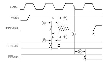
Figure 11-10. Background Debug Mode Serial Port Timing
