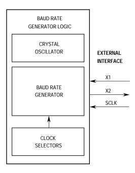
Figure 7-3. Baud Rate Generator Block Diagram
