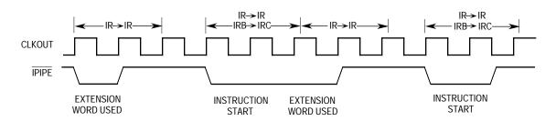
Figure 5-29. Instruction Pipeline Timing Diagram
