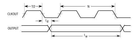
Figure 10-12. Signal Width Specifications
