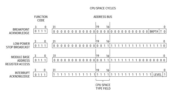
Figure 3-10. CPU Space Address Encoding
