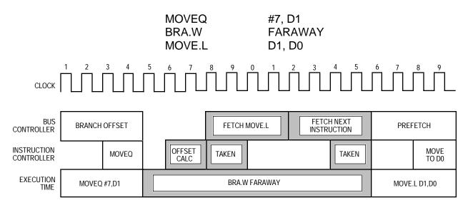
Figure 5-36. Example 3—Branch Negative Tail
