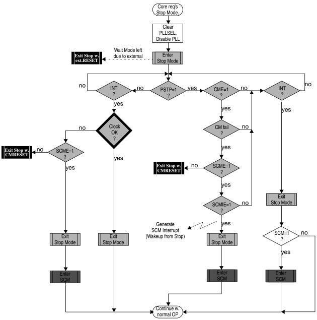
Figure 4-24. Stop Mode Entry/Exit Sequence
