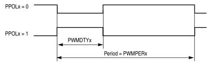
Figure 12-36. PWM Left Aligned Output Waveform
