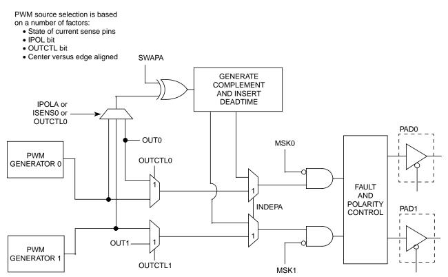
Figure 11-2. Detail of Mux, Swap, and Deadtime Functions
