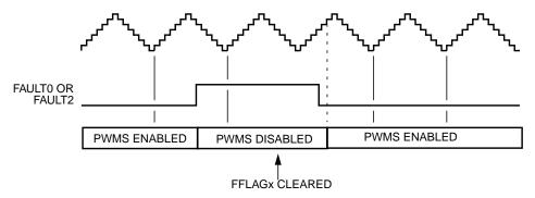
Figure 11-77. Manual Fault Clearing (Faults 0 and 2) - QSMP = 00
