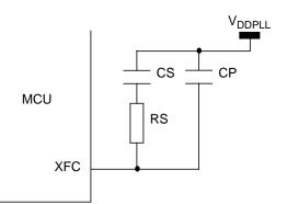
Figure 4-2. PLL Loop Filter Connections
