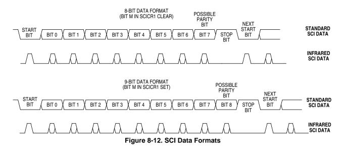
Each data character is contained in a frame that includes a start bit, eight or nine data bits, and a stop bit. Clearing the M bit in SCI control register 1 configures the SCI for 8-bit data characters. A frame with eight data bits has a total of 10 bits. Setting the M bit configures the SCI for nine-bit data characters. A frame with nine data bits has a total of 11 bits
