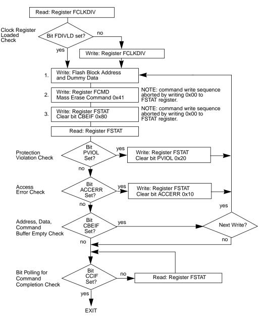
Figure 2-28. Example Mass Erase Command Flow
