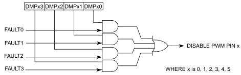
Figure 11-15. Fault Decoder
