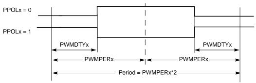
Figure 12-38. PWM Center Aligned Output Waveform
