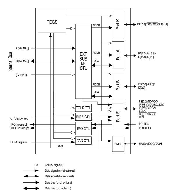
Figure 18-1. MEBI Block Diagram
