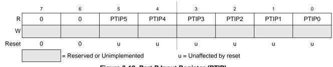
Figure 3-18. Port P Input Register (PTIP)
