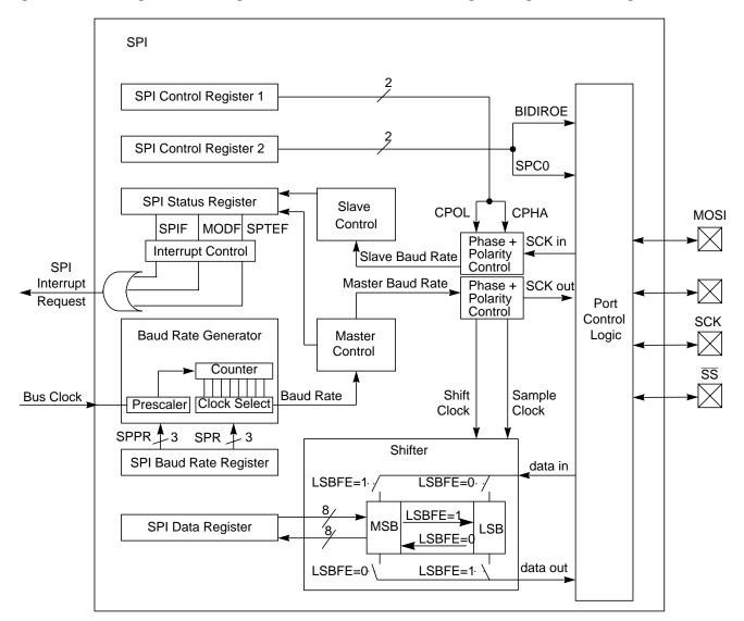
Figure 9-1. SPI Block Diagram
