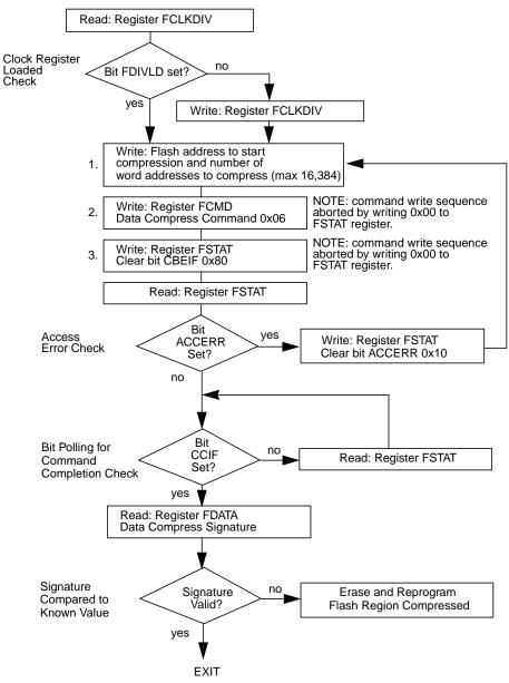
Figure 2-24. Example Data Compress Command Flow
