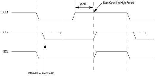
Figure 10-11. IIC-Bus Clock Synchronization
