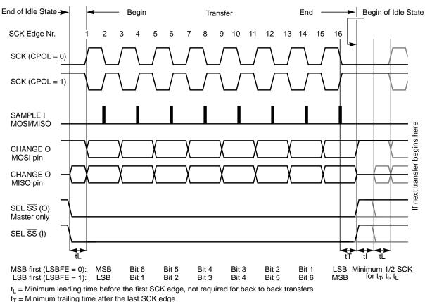
$t_1$  = Minimum idling time between transfers (minimum  $\overline{SS}$  high time), not required for back to back transfers
