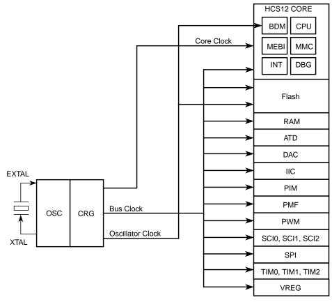
Figure 1-7. Clock Connections
