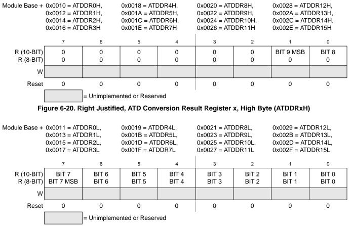
Figure 6-21. Right Justified, ATD Conversion Result Register x, Low Byte (ATDDRxL)
