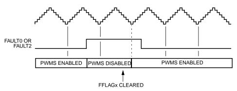
Figure 11-78. Manual Fault Clearing (Faults 0 and 2) — QSMP = 01, 10, or 11
