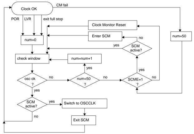
Figure 4-20. Sequence for Clock Quality Check
