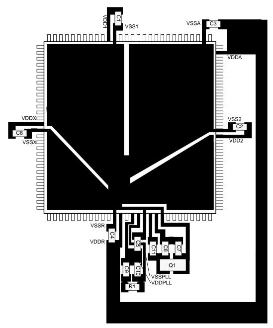
Figure 1-8. Recommended PCB Layout (112-LQFP)
