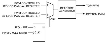
Figure 11-54. Internal Correction Logic when ISENS = 01
