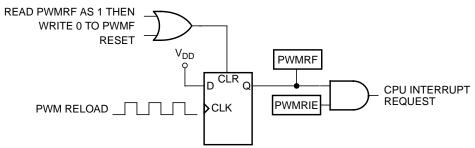
Figure 11-67. PWMRF Reload Interrupt Request
