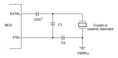
1. Due to the nature of a translated ground Colpitts oscillator a DC voltage bias is applied to the crystal. Please contact the crystal manufacturer for crystal DC
