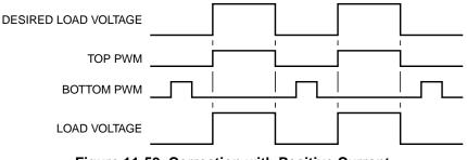
Figure 11-59. Correction with Positive Current
