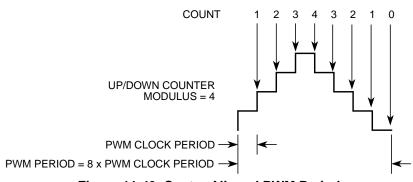
Figure 11-43. Center-Aligned PWM Period
