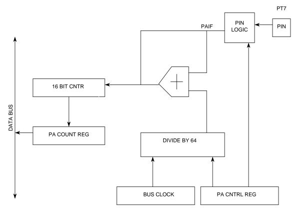
Figure 13-22. Pulse Accumulator System Block Diagram
