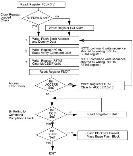
Figure 2-23. Example Erase Verify Command Flow
