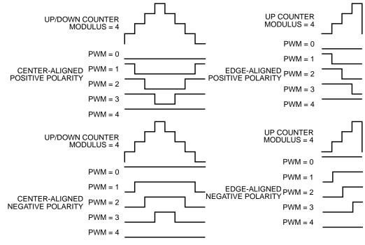
Figure 11-61. PWM Polarity
