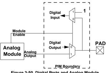
Figure 3-50. Digital Ports and Analog Module
