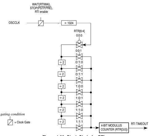
Figure 4-22. Clock Chain for RTI
