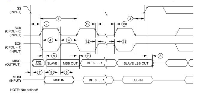
Figure A-8. SPI Slave Timing (CPHA = 1)
