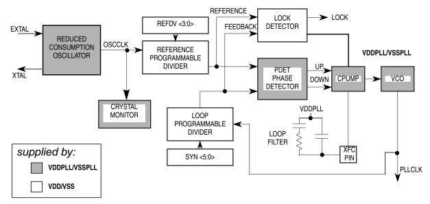
Figure 4-16. PLL Functional Diagram
