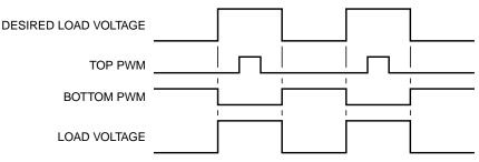
Figure 11-60. Correction with Negative Current
