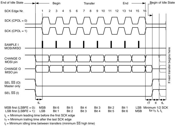
$t_{l}$ ,  $t_{T}$ , and  $t_{l}$  are guaranteed for the master mode and required for the slave mode.
