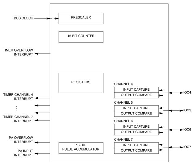
Figure 13-1. Timer Block Diagram
