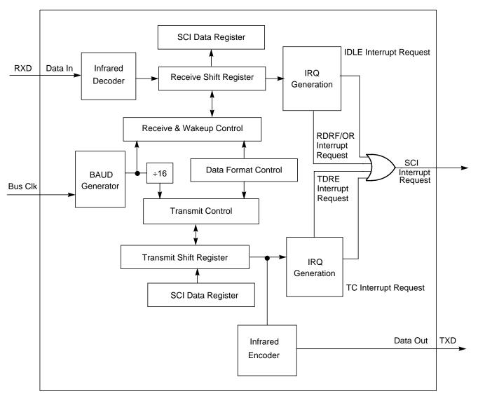
Figure 8-1. SCI Block Diagram
