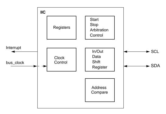
Figure 10-1. IIC Block Diagram
