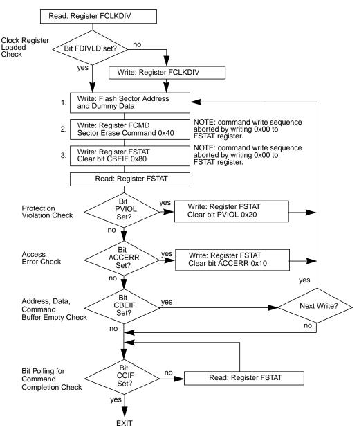
Figure 2-27. Example Sector Erase Command Flow
