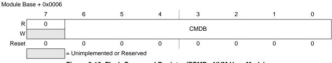
Figure 2-12. Flash Command Register (FCMD - NVM User Mode)
