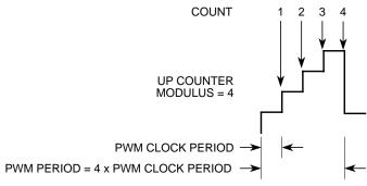
Figure 11-44. Edge-Aligned PWM Period
