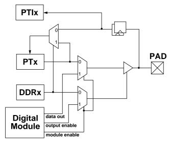
Figure 3-49. Illustration of I/O Pin Functionality
