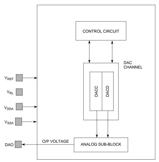
Figure 7-1. DAC8B1C Functional Block Diagram
