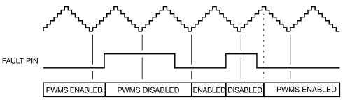
Figure 11-76. Automatic Fault Clearing
