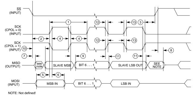
In Figure A-7 the timing diagram for slave mode with transmission format CPHA = 0 is depicted.
