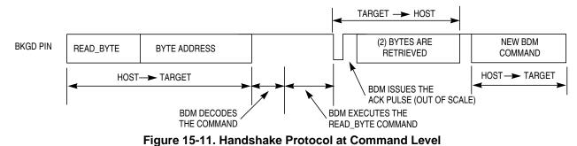
Differently from the normal bit transfer (where the host initiates the transmission), the serial interface ACK handshake pulse is initiated by the target MCU by issuing a falling edge in the BKGD pin. The hardware
