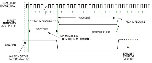
Figure 15-10. Target Acknowledge Pulse (ACK)
