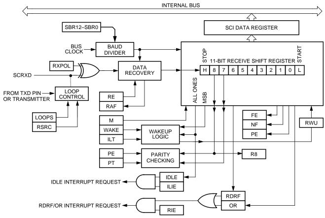
Figure 8-14. SCI Receiver Block Diagram
