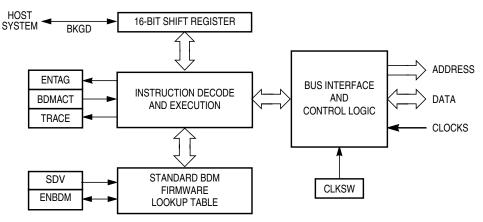
Figure 15-1. BDM Block Diagram
