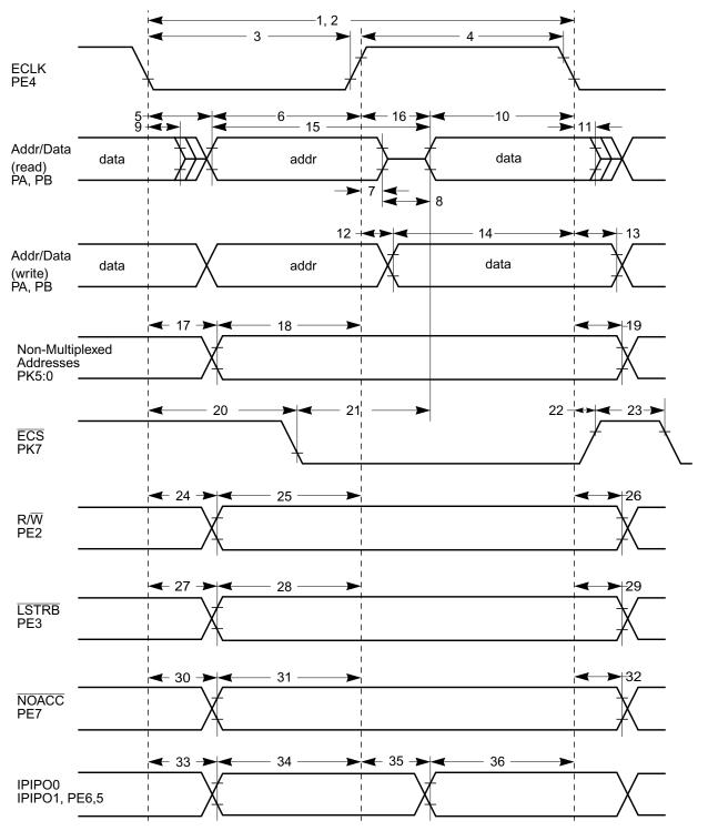
Figure A-10. General External Bus Timing
