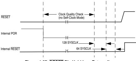
Figure 4-27. RESET Pin Held Low Externally
