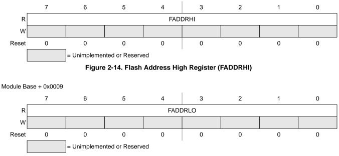
Figure 2-15. Flash Address Low Register (FADDRLO)
