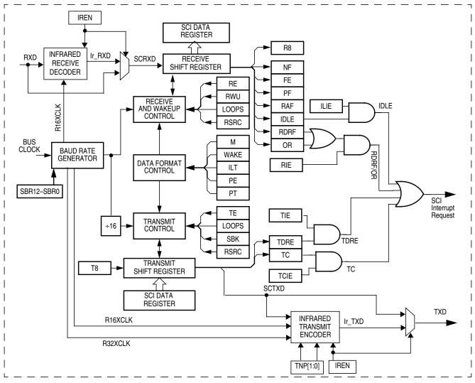
Figure 8-11. Detailed SCI Block Diagram
