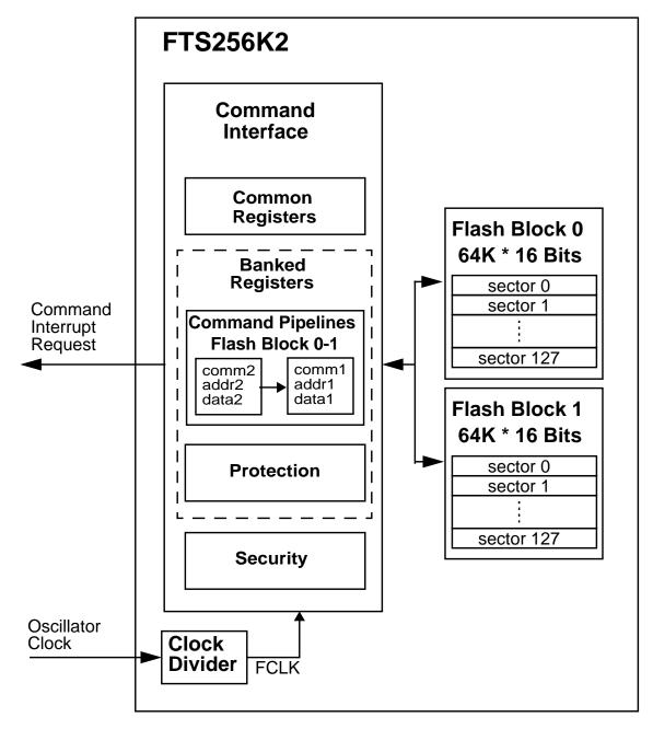
Figure 2-1. FTS256K2 Block Diagram
