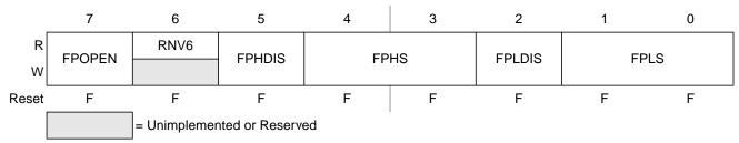
Figure 2-8. Flash Protection Register (FPROT)
