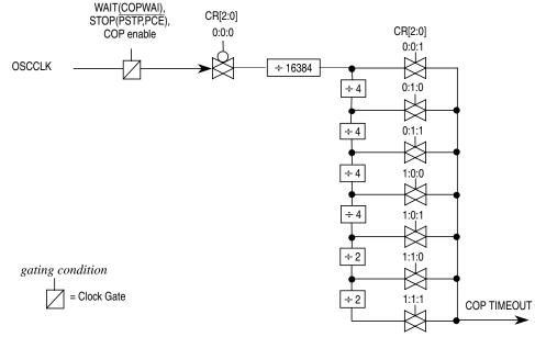
Figure 4-21. Clock Chain for COP
