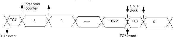
Figure 13-21. The TCNT cycle diagram under TCRE=1 condition
