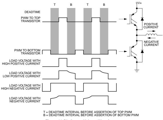
Figure 11-56. Output Voltage Waveforms
