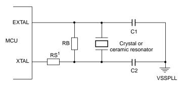
1. Rs can be zero (shorted) when use with higher frequency crystals. Refer to manufacturer's data.
