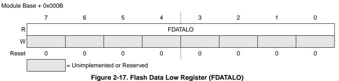
All FDATAHI and FDATALO bits are readable but are not writable. After an array write as part of a
