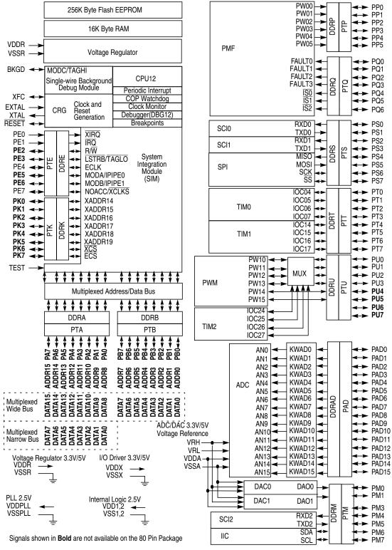
Figure 1-1. MC9S12E256 Block Diagram
