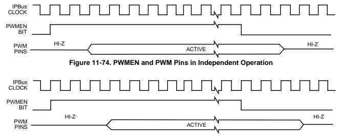
Figure 11-75. PWMEN and PWM Pins in Complementary Operation
