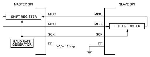
Figure 9-8. Master/Slave Transfer Block Diagram
