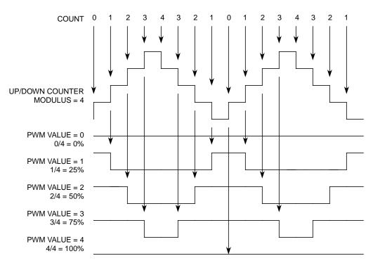
Figure 11-45. Center-Aligned PWM Pulse Width
