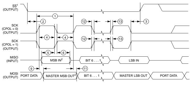
In Figure A-6 the timing diagram for master mode with transmission format CPHA=1 is depicted.
