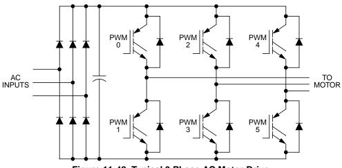
Figure 11-48. Typical 3 Phase AC Motor Drive
