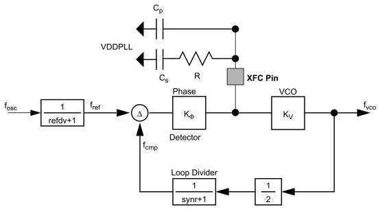
Figure A-2. Basic PLL Functional Diagram
