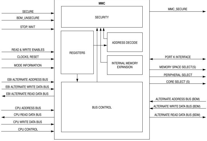
Figure 19-1. MMC Block Diagram
