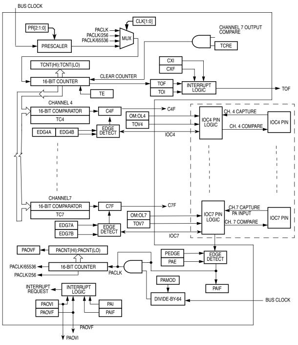
Figure 13-20. Detailed Timer Block Diagram
