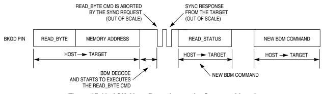
Figure 15-12. ACK Abort Procedure at the Command Level
