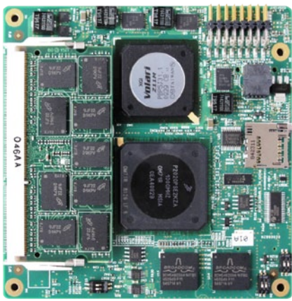
Figure 1: Emerson Network Power COM Express™ compatible module based on the QorIQ P2020 processor
