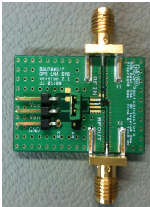
Fig 1. BGU7008 GPS LNA evaluation board
