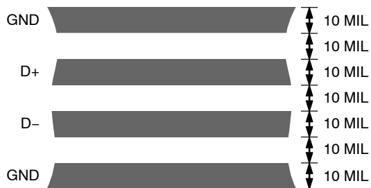
Figure 19. Arrangement of Signal Tracks
