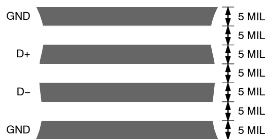
Figure 28. Arrangement of Signal Tracks
