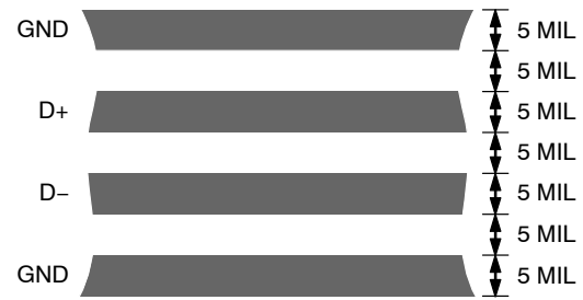
Figure 22. Typical Arrangement of Signal Tracks
