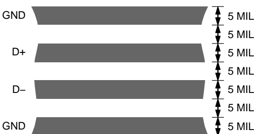
Figure 21. Typical Arrangement of Signal Tracks
