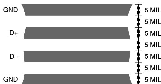
Figure 16. Arrangement of Signal Tracks
