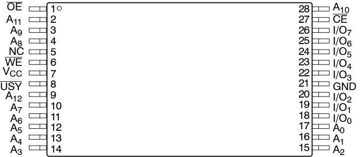
TSOP Package (8 mm x 13.4 mm) (H13)
