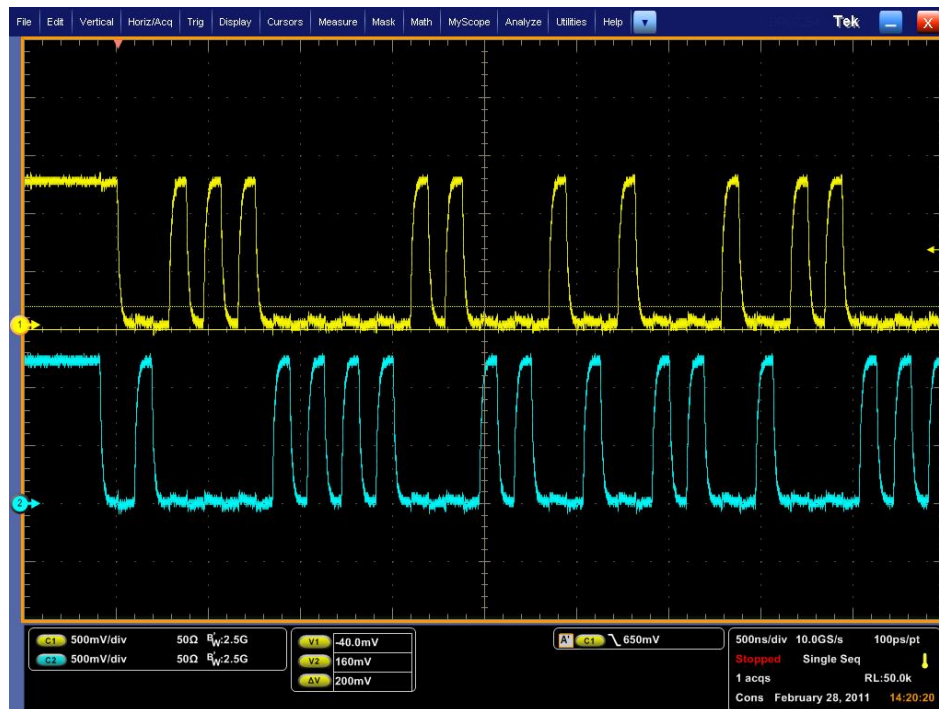
Figure 8. EMI4182 MIPI D-PHY LP Mode Measured Results
