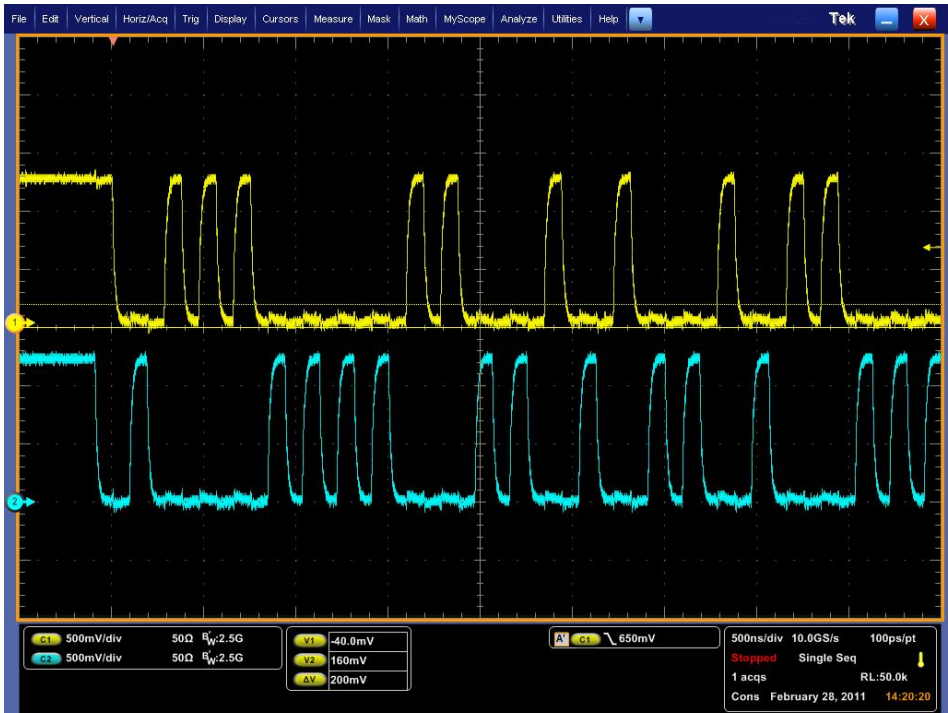
Figure 8. EMI4182MU MIPI D-PHY LP Mode Measured Results
