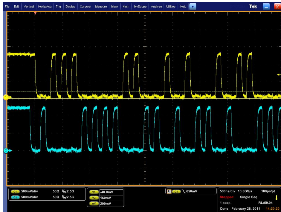
Figure 8. EMI4184 MIPI D-PHY LP Mode Measured Results
