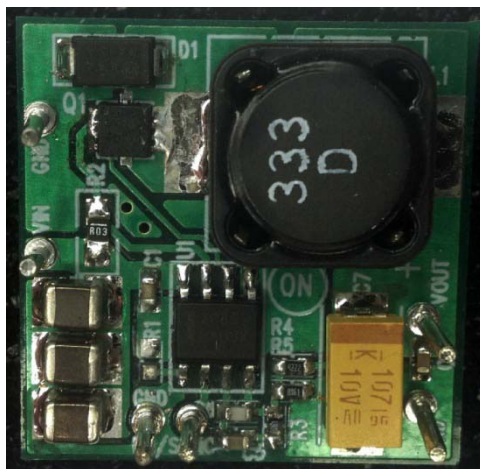
Figure 1. NCV8852GEVB Board Picture
