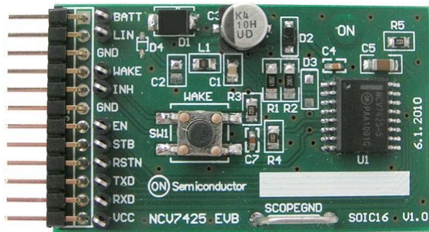
Figure 12. NCV7425EVB PCB Top Side View
