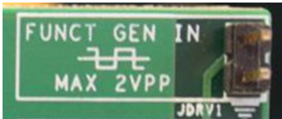
Figure 9. Internal Drive (Square Wave Input)
