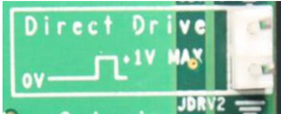
Figure 7. Direct Drive (Drives DLT Load Amps Directly)
