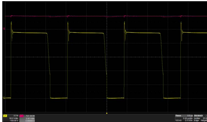
Figure 5. QR (1 st Valley) Operation @ 45 W / 115 V rms
