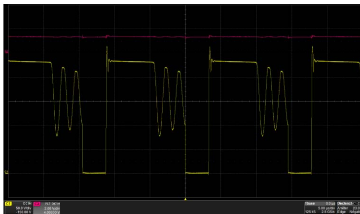
Figure 7. 3 rd Valley Operation @ 25 W / 115 V rms
