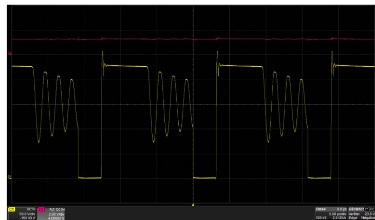
Figure 8. 4 th Valley Operation @ 20 W / 115 V rms
