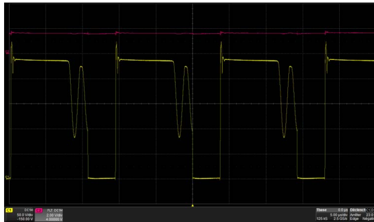
Figure 6. 2 nd Valley Operation @ 35 W / 115 V rms
