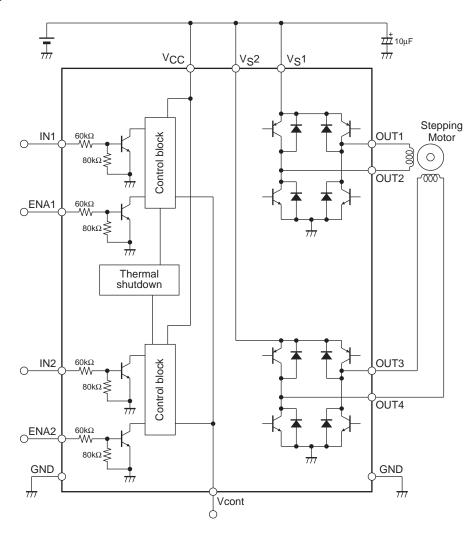
Note: As long as the voltages applied to  $V_{CC}$ ,  $V_{S1}$ ,  $V_{S2}$ , ENA1, ENA2, IN1, and IN2 are within the limits set by the absolute maximum ratings, there are no restrictions on the relationship of each voltage level in comparison with the others (regarding which is higher or lower). (ex.  $V_{CC} = 3V$ ,  $V_{S1}$ ,  $V_{S1}$ ,  $V_{S2}$ ,  $V_{S1}$ ,  $V_{S2}$ ,  $V_{S3}$ ,  $V_{S4}$ ,  $V_{$
