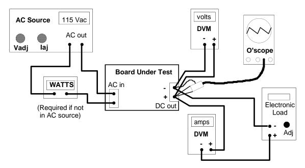
NOTE: The outputs of this board <u>are not isolated</u> from the AC input, so use precaution when using electronic loads or when touching or probing the board.
