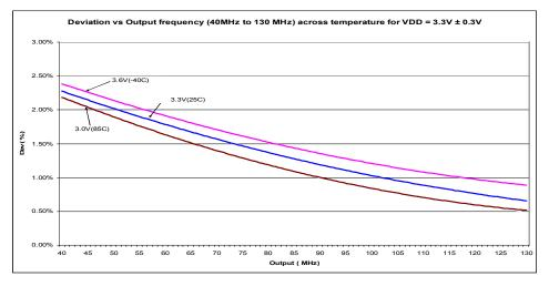
Note: Transition band is 30MHz to 34MHz for VDD=2.5V ± 5%, across -40°C to +85C. Deviation in this band is 1.93% ± 37%. Transition band is 30MHz to 39MHz for VDD=3.3V ± 0.3V, across -40°C to +85C. Deviation in this band is 1.8% ± 45%.
