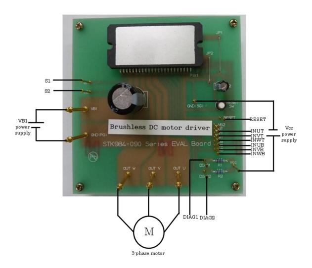
[Supply Voltage] VB1 (8 to 18V): Power Supply for 3-phase motor & Driver IC Vcc (5V): Pull up Power Supply for DIAG1, DIAG2
