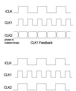
Using CLK1 as feedback will always result in synchronized rising edges between ICLK and CLK1 if CLK1 is used as feedback. CLK2 could be a falling edge compared to ICLK. Therefore, wherever possible, it is recommended to use CLK2 for feedback, which will synchronize the rising edges of all three clocks.
