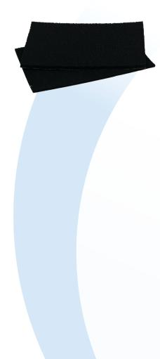
Part Number 5206 is a lightweight lossy foam sheet absorber, which achieves a broad frequency range of dielectric loss through a carbon coating. 5206 has similar performance to PN5103, but has no sulfur in its formulation. Surfactants used in industry carbon latex coatings have small amounts of sulfur in them. This can cause corrosion inside of electronic housings in certain application. PN 5206 has no sulfur in the coating and eliminates this problem.
