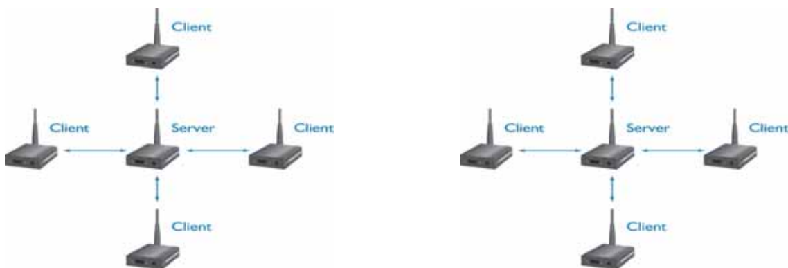
Figure 9- Multiple Networks of Point-to-Multipoint CL4424s
