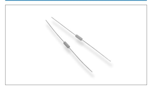
The TE Connectivity Series of Zerohm links are available in two standard case sizes and element types. No end caps are used for the steel element, terminations are welded directly on to the steel slug. For the Ceramic elements, tinned copper wire leads are welded onto end caps. This manufacturing process allows for very low resistance values to be achieved. The slugs are then finished by applying three coats of light brown epoxy resin.
