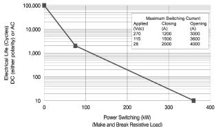
\*Failure Mode: Dielectric withstand voltage test @ 2000 Vdc, power terminal to terminal, leakage exceeds 1.0 mA. Current carry: 500 A @ 25°C. Derate 2.5 A/°C to 350 A @ 85°C for still air, no heat sink, AWG# 00 conductor.
