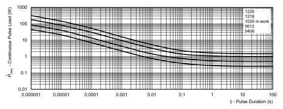
Maximum pulse load, continuous pulses; applicable if  $\bar{P} \leq P(v_{amb})$  and  $\hat{U} \leq \hat{U}_{max}$ ; for permissible resistance change equivalent to 8000 h operation
