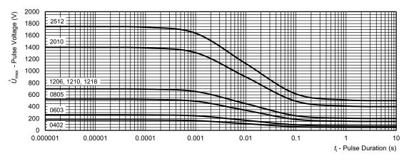
Maximum pulse voltage, single and continuous pulses; applicable if  $\hat{P} \leq \hat{P}_{max}$ ; for permissible resistance change equivalent to 8000 h operation
