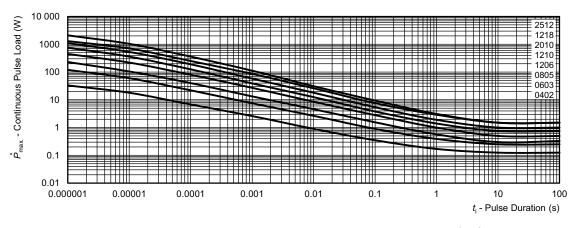
Maximum pulse load, continuous pulses; applicable if  $\bar{P} \le P(\theta_{amb})$  and  $\hat{U} \le \hat{U}_{max}$ ; for permissible resistance change equivalent to 8000 h operation
