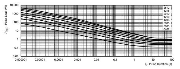
Maximum pulse load, single pulse; applicable if  $\bar{P} \rightarrow 0$  and n < 1000 and  $\hat{U} \le \hat{U}_{max}$ ; for permissible resistance change equivalent to 8000 h operation
