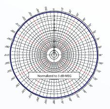
Azimuth Pattern (X,Y, or E-plane)
