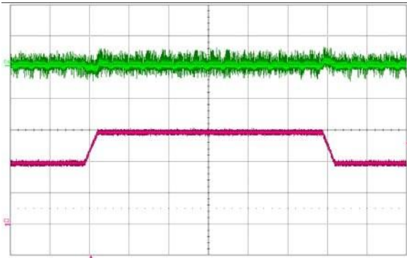
Figure 11. Output voltage response to load current step change (10 A – 15 A – 10 A) at V_{in} = 48 V. Top trace: output voltage (100 mV/div.) Bottom: load current (5 A/div.). Current slew rate: 0.1 \text{ A}/\mu\text{s} . Time scale: 200 \mu\text{s}/\text{div} . C_o = 10 \mu\text{F} tantalum + 1 \mu\text{F} ceramic
