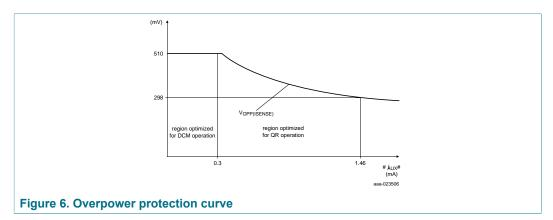
During system start-up, the maximum time-out period is lowered to 38.4 ms. When the output voltage is within its regulation level, the maximum time-out period returns to 192 ms, limiting the output power to a minimum at a shorted output. Shortening the overpower timer ensures that the input power of the system is limited to < 5 W at a shorted output.
