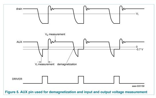
When the external MOSFET is switched on, the voltage at the auxiliary windings reflects the input voltage. The AUX pin is clamped to -0.7 V. The output current is a measure of the input voltage. This current value is internally used to set the overpower limit on  $V_{\text{sense(ipk)}}$ . The demagnetization and output voltages are measured as a voltage on the AUX pin. In this way, the input voltage measurement and OVP can be adjusted independently.
