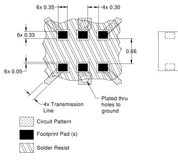
Dimensions are in Millimeters Mounting Footprint
