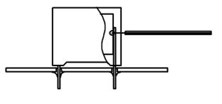
Temperature monitored inside the capacitor.
