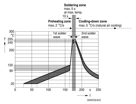
**Important note:** Temperatures of all preheat stages and the solder bath must be strictly controlled.
