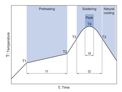
Preheating Soldering Peak Temp. Temp. Time Time Temp. Time T1 T2 T4 Т3 t3 150°C 180°C 60 to 120s 230°C 250°C 30s 5s
