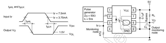
(\*) CL is approximately 15pF which includes probe and stray wiring capacitance.
