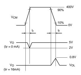
$$CM_{H}=\frac{320\left(V\right)}{t_{f}\left(\mu s\right)},CM_{L}=\frac{320\left(V\right)}{t_{f}\left(\mu s\right)}$$
