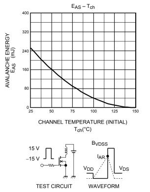
$\begin{aligned} R_G &= 25~\Omega \\ V_{DD} &= 90~V,~L = 6.04~mH \end{aligned} \qquad E_{AS} &= \frac{1}{2} \cdot L \cdot I^2 \cdot \left( \frac{BVDSS}{BVDSS - VDD} \right) \end{aligned}$
