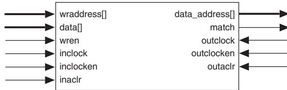
Figure 23. APEX 20KC CAM Block Diagram
