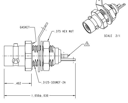
4. SUBMINIATURE TRIAXIAL SOLDER POT BULKHEAD MOUNT 3-LUG RECEPTACLE (TPS STYLE)
