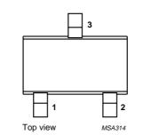
Fig.1 Simplified outline (SC59) and pin configuration.
