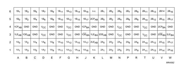
Fig.1 Pin configuration.
