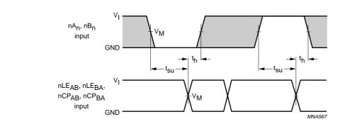
The shaded areas indicate when the input is permitted to change for predictable output performance.
