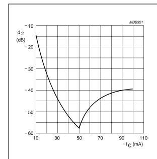
$V_{CE} = -10 \text{ V; } V_o = 50 \text{ dBmV; } T_{amb} = 25 \text{ °C;}$   $f_{(p+q)} = 810 \text{ MHz.}$
